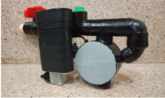
Fig. 3. The electricity generating water faucet with three-inflow pipes generator.
